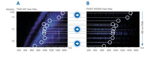
**The principle of PASEF acquisition:** Peptide ions are separated using trapped ion mobility spectrometry, eluted (~ 100 ms) and detected in the QTOF, generating the TIMS MS heat map (A). For acquisition of PASEF MS/MS spectra (B) the same TIMS separation is used with the quadrupole isolating a certain ion species only during its mobility elution time and immediately shifting to next precursor. Parent and fragment spectra are aligned by mobility values.
