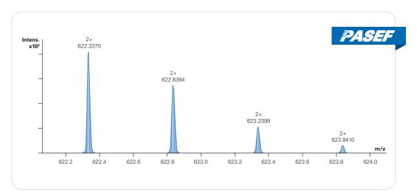
High mass resolving power independent of sequencing speed. Measurements were performed with a resolving power of 50,000 (FWHM @ m/z 1222)
