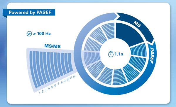
**Parallel accumulation serial fragmentation (PASEF) cycle time:** By synchronizing the quadrupole with the TIMS elution time, an average of 12 precursors can be fragmented within a 100 ms timescale. Intelligent software targets low-level precursors multiple times for PASEF MS/MS fragmentation.
