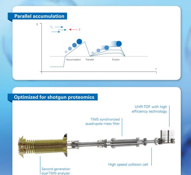
**Schematic of the timsTOF Pro.** All ion optics have been optimized to enhance proteomics performance, including an enhanced quadrupole synchronized with the TIMS analyzer to enable time-focusing, a high speed collision cell and an actively cooled temperature controlled flight tube.
