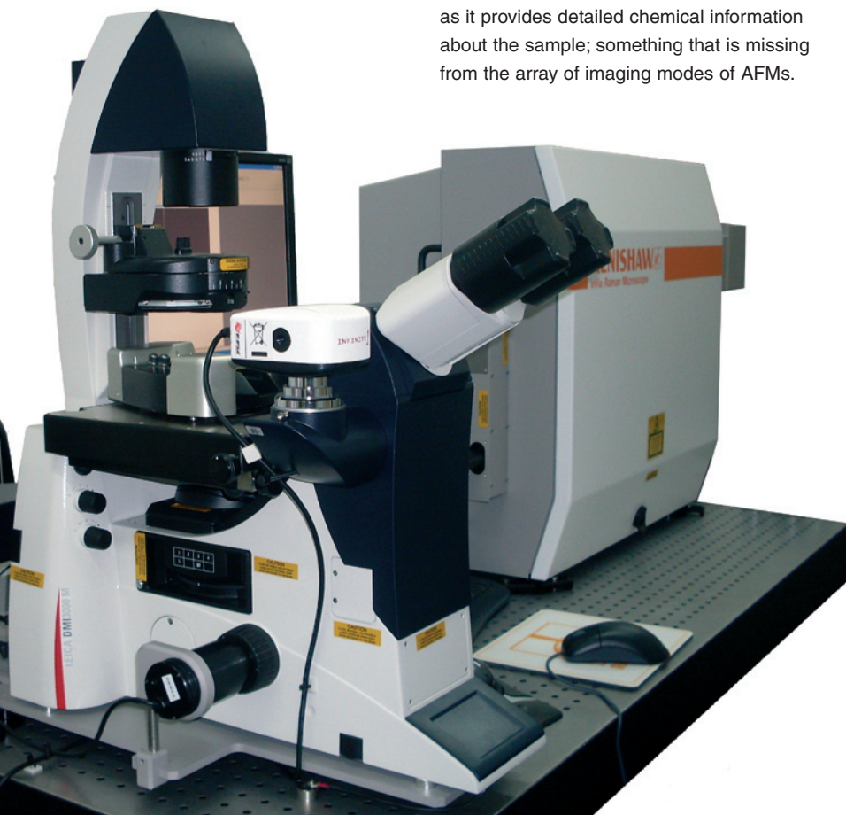
Veeco BioScope II AFM coupled to an inVia Raman microscope.
