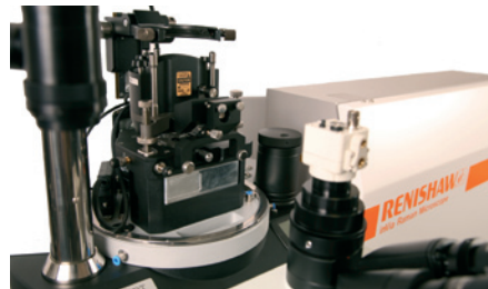
An NT-MDT NTEGRA AFM system with direct optical coupling to an inVia Raman microscope.
