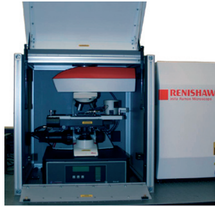
inVia Raman microscope with a Nanonics MV4000 AFM system housed in a custom acoustic enclosure.
