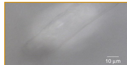
Photograph of a dull inclusion in a polypropylene film
