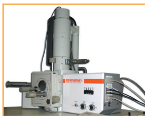
The structural and chemical analyser fitted to an SEM column.
