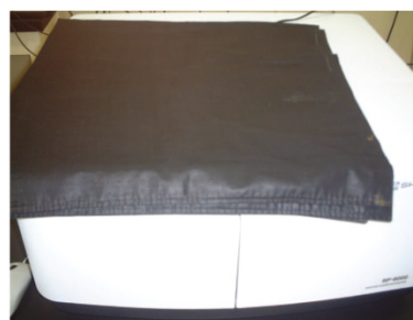
图 3 加盖遮光布进行测定 Measurements with Sample Compartment Covered with Blackout Cloth
