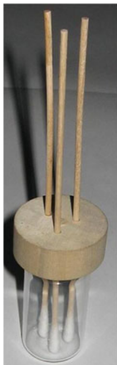
Figure 2. Fixture for simultaneous sampling with three cotton swabs.
