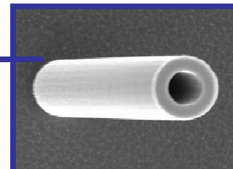
Nozzle dimensions: 5.5  $\mu\text{m}$  ID x 28  $\mu\text{m}$  OD x 55  $\mu\text{m}$  height
