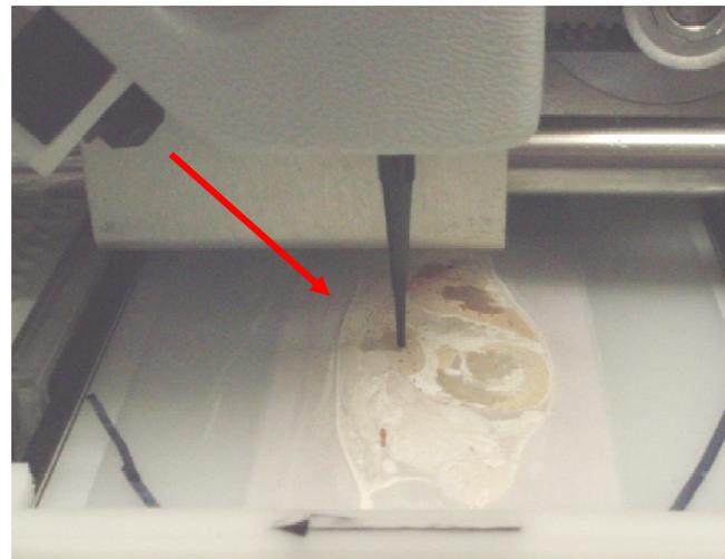
On board camera system is available for AB/Sciex MS instruments with LESA<sup>Clarity</sup>
