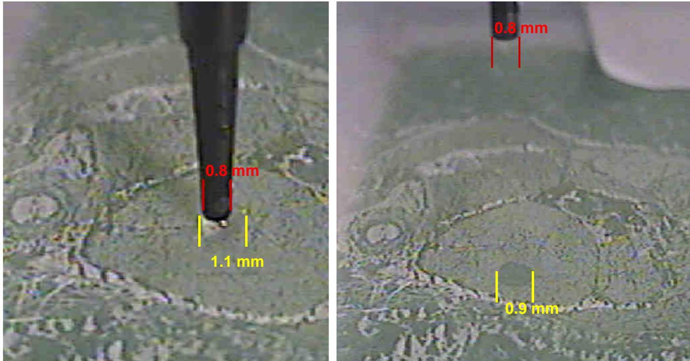
1.2  $\mu\text{L}$  extraction solvent pick up, 0.7  $\mu\text{L}$  dispense on target, 0.9  $\mu\text{L}$  aspirate from target
