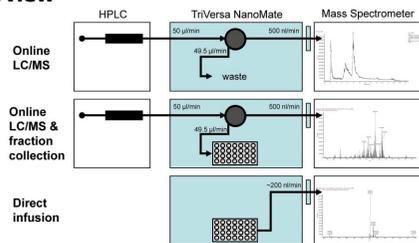
**HPLC:** Lipid extracts were analyzed by a Dionex LC system equipped with a FAMOS autosampler. Samples were kept at 10°C and injection volume was 0.5-1 µl. Chromatographic separation of lipids was achieved using a normal phase YMC-Pack PVA-Sil column (150x1.0 mm) and a ternary gradient composed of A: Hexane/IPA (98/2); B: MTBE/IPA (45/55); C: MeOH; where B and C contained 5 mM AA. The flow rate was 50 µL/min.
