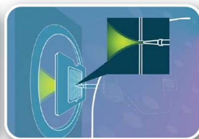
The solvent is retracted into the pipette tip and is analyzed by chip-based infusion.
