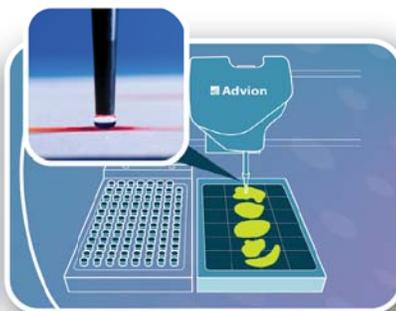
The robot brings the extraction solvent into contact with the surface of the sample. The analyte is extracted from the surface.
