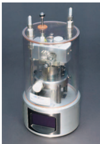
Figure 10a. (a.) The Atmospheric Hood for the MultiMode SPM allows control of the gaseous imaging environment to vary humidity or image under inert gases.
