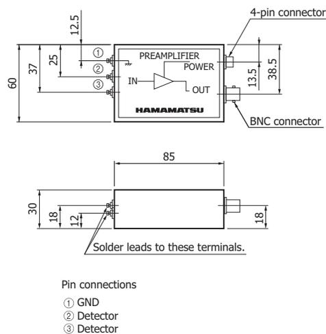
Note: Socket for lead attachment is not provided.
