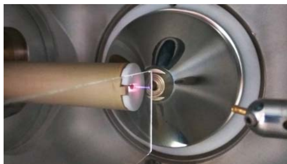
Figure 2: Position of the DBDI source (left) with respect to the MS inlet.
