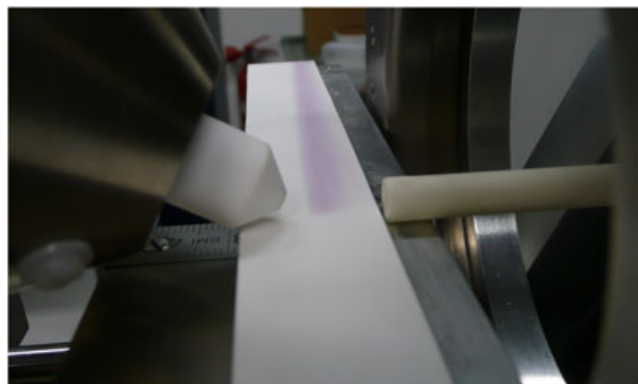
Figure 5. Experimental setup with the DART ion source with the desorption at an angle option (DART SVP-A). The visualization was performed in real-time using the substrate treated with the 2-naphthol sulfuric acid reagent.
