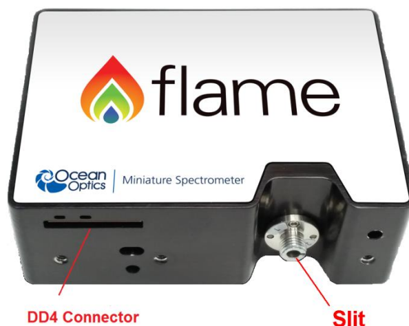
Location of Flame Accessory Connector
