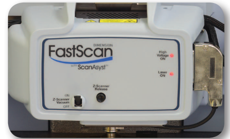
Scanner Resonant Frequency X-Y: 2.70kHz, Z: >50kHz.
