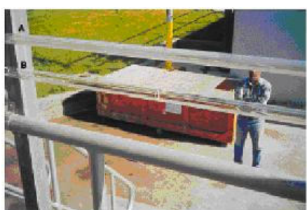
Fig. 11. UV lamp quartz tubes; A is fouled tube; B is acid-cleaned tube
