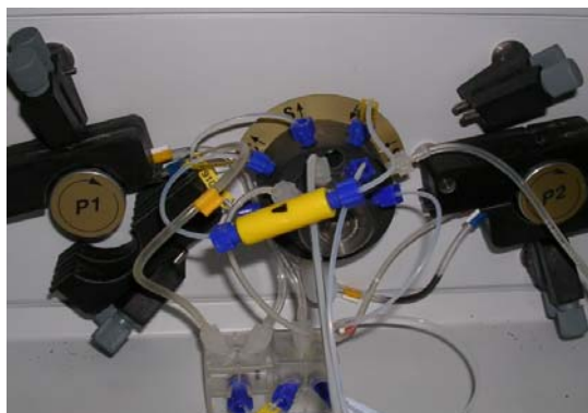
Figure 2. FIAS-400 and activated alumina mini column (yellow)
