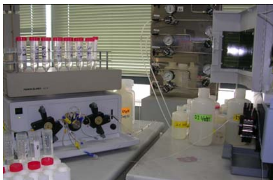
Figure 1. FI-ICP-OES with FIAS-400, Autosampler 91 and Optima 5300 DV ICP-OES
