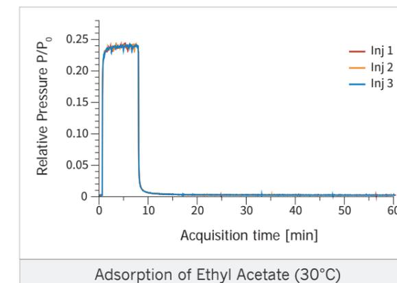
The automated injection system provides a continuous and controlled flow of probe molecules thus avoiding successive injections. In this example, 60 minutes are sufficient to get several hundred experimental points. Moreover, this innovative method leads to a repeatability level which was not achievable before.
