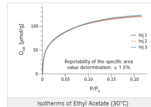
When determining the specific area value using the Finite Concentration method and the adsorption isotherms, the mean standard deviation computed after three measurements does not exceed 1.5%.
