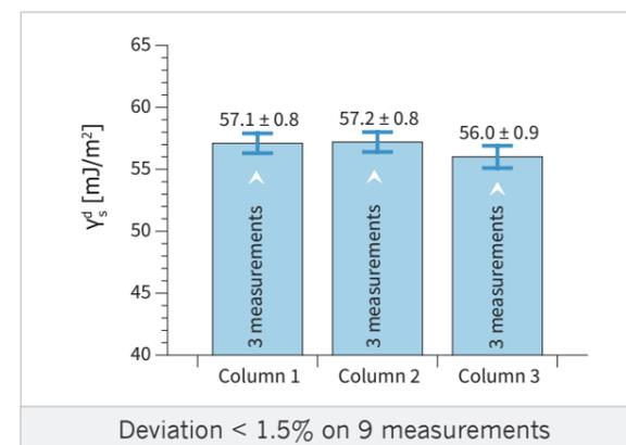
When computing the dispersive component of the surface energy through the Infinite Dilution method, in 3 different columns and with 3 replicas each time, an average standard deviation of less than 1% is observed.
