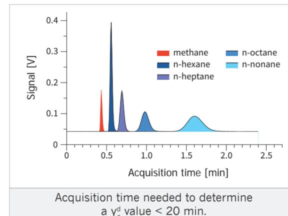
The above example shows that twenty minutes are sufficient to get the retention times of a homologous series of n-alkanes and then the resultant dispersive component of the surface energy. Indeed, the device is able to stop the analysis once the first probe has been fully detected and inject the next one without any human intervention. This allows the operator to handle other tasks within this automatic cycle.
