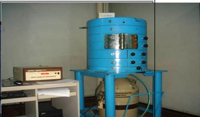
高纯锗γ能谱仪(γ(Spectrometer for Cs, U, Th and Ra' s γ-nuclide analysis)
